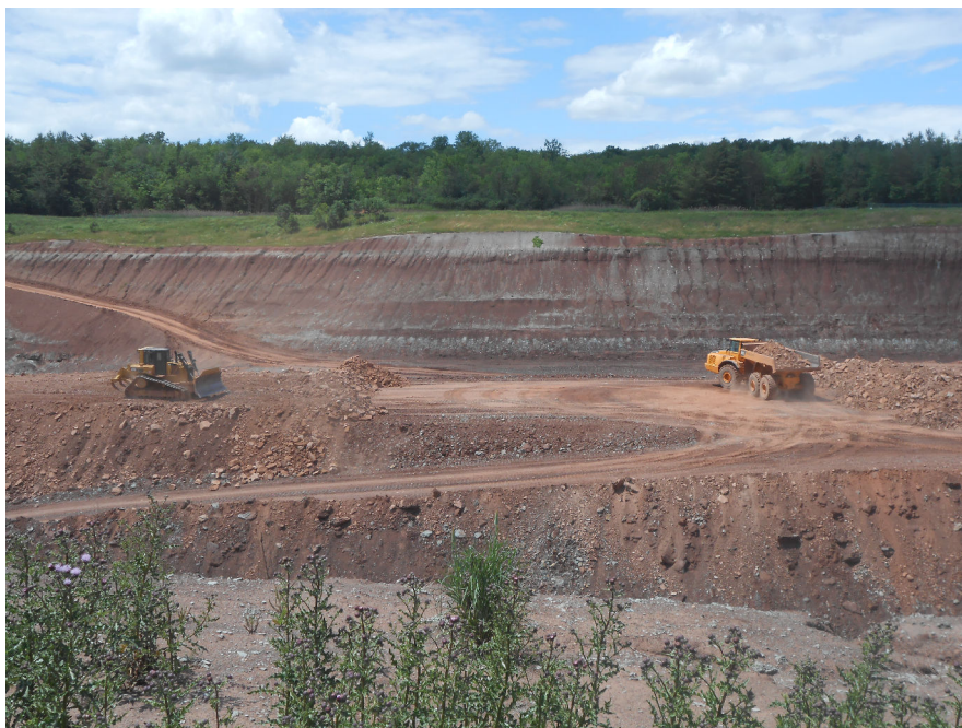
Photo 3. The Cheltenham Quarry of Brampton Brick Ltd. showing the red shale of the Queenston Formation with minor interbeds of blue, carbonate-rich shale. The blue material is incorporated and homogenized with the red, iron oxide-rich material to ensure proper firing of the bricks. Photo by P.S. LeBaron, June 2017 (Resident Geologist’s Files, Southern Ontario Region, Tweed).
