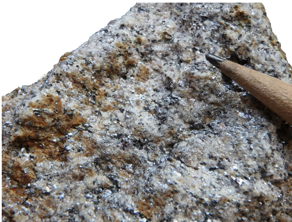
Photo 10. Sample BM-18-11 showing disseminated, grey graphite flakes in quartz-rich metasedimentary rock; white, highly reflective grains are muscovite and/or phlogopite. Graphite content is 3.47% (analysis by Activation Laboratories; see Table 10).
