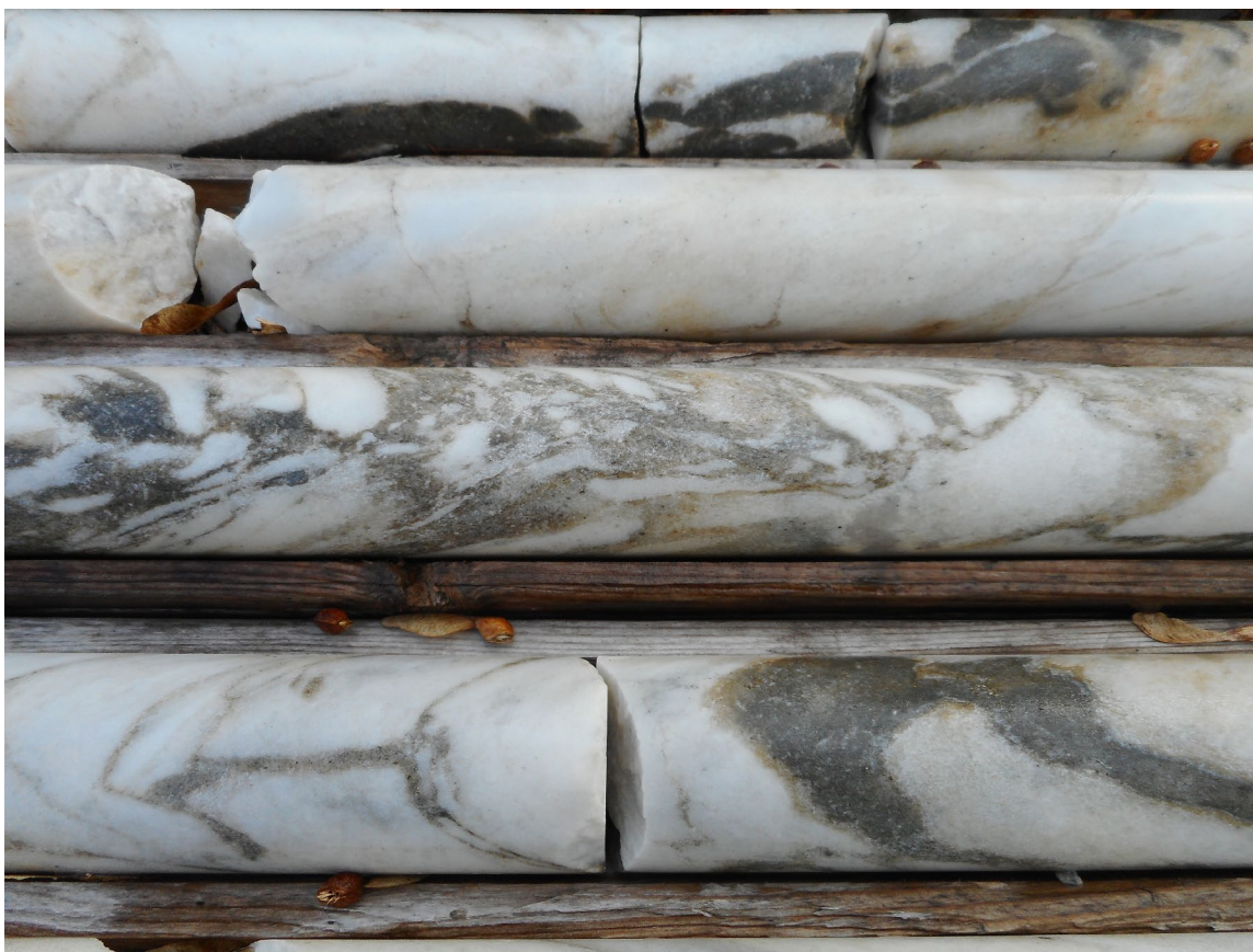
Photo 10. White marble breccia fragments with dark green serpentine matrix and veining, Canada Talc Mine.
