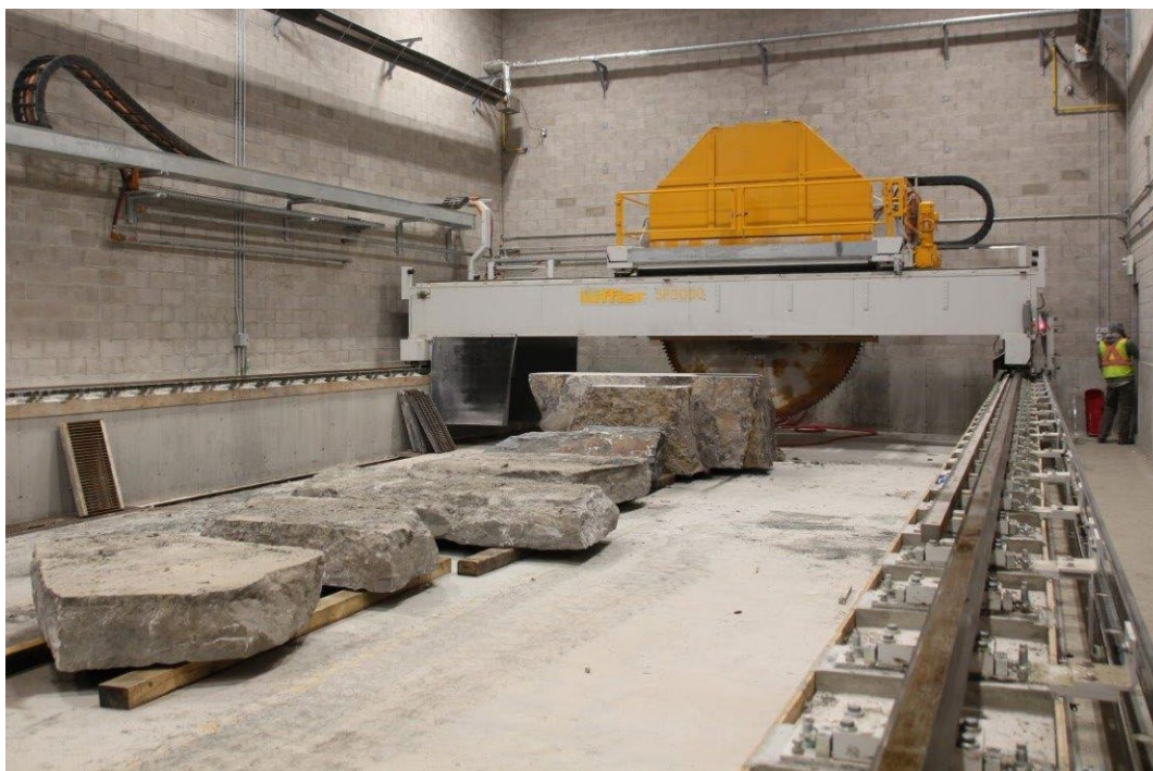
Photo 5. Slab saw, 118-inch diameter, Drain Bros. Excavating Ltd. stone processing facility, Havelock. Photo supplied by D. Corcoran (Drain Bros. Excavating Ltd., February 2018).
