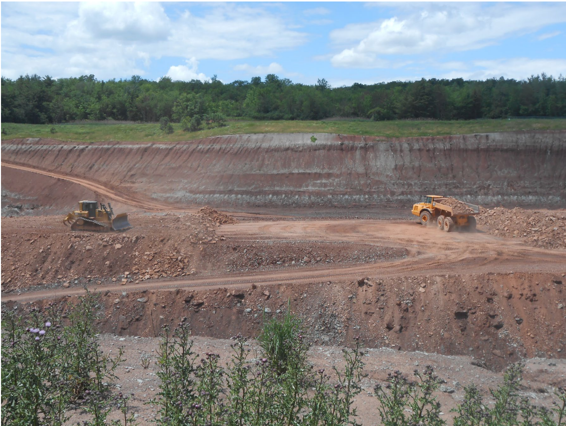
Photo 3. The Cheltenham Quarry of Brampton Brick Ltd. Red shale of the Queenston Formation with minor interbeds of blue, carbonate-rich shale. The blue material is incorporated and homogenized with the red, iron oxide-rich material to ensure proper firing of the bricks. Photo by P.S. LeBaron, June 2017 (Resident Geologist's Files, Southern Ontario Region, Tweed).
