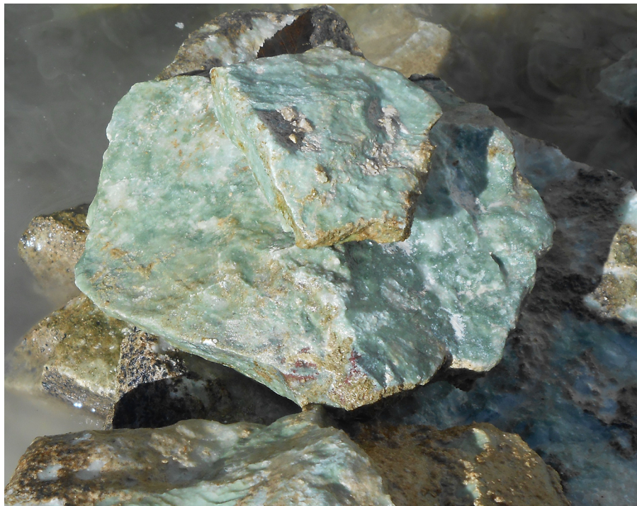
Photo 6. Green, tremolitic marble (sample TW-14-01) collected from the Upper Canada Stone Company Ltd. quarry, Huntingdon Township; white mottling is calcitic marble, sample width 16 cm.
