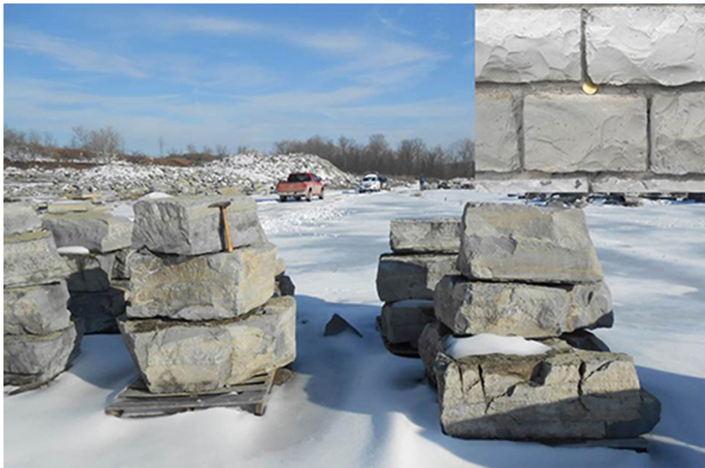
Photo 1. Thickly bedded, micritic limestone of the Gull River Formation, Petworth Quarry; hammer, for scale, is 35 cm long. Inset (at top right) shows Petworth stone in a building wall (McDonald’s restaurant, Division St., Kingston), exhibiting the white patina typical of Kingston limestone, developed during the 30 years since installation.
